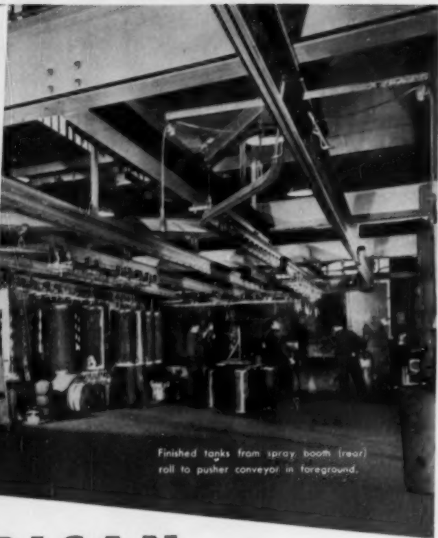
American MonoRail System for finishing water conditioner tanks.
